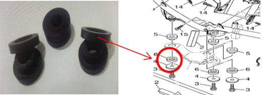
damper handlebar damage
