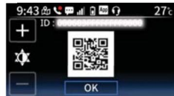
This module contains a QR code with the CCU's unit identification number. The “ $\wedge$ ”/“ $\vee$ ” switches control the brightness of the QR code. Short press the “ $\checkmark$ ” switch to return to the previous menu.
