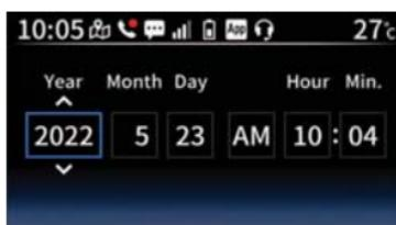
To manually adjust the clock, Short press the “^”/“▼” switches to adjust the highlighted item up/down. Short press the “✓” switch to set the item and continue to the next item in line. After the last item is set, select “OK” and the display will return to the previous menu.
