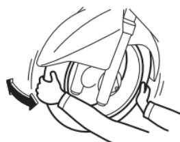
The front and rear wheel bearings must be checked at the intervals specified in the periodic maintenance and lubrication chart. If there is play in the wheel hub or if the wheel does not turn smoothly, have a Yamaha dealer check the wheel bearings.
