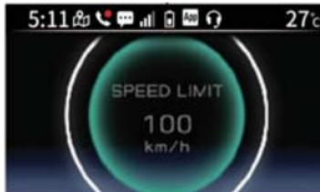
The speed limit on the road currently being traveled on is indicated with text and by the outer circle. The inner circle
