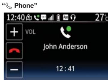
Selecting this module opens an active call screen. The contact name and call time are displayed.
