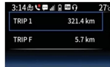
This module allows reset of the tripometers on the main display. Short press the “ $\wedge$ ”/“ $\vee$ ” switches to highlight an item. Long press the “ $\checkmark$ ” switch to reset the item. Confirm by selecting “OK”.
