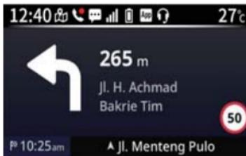
Short press the "↙" switch to open the menu system and navigate to "🚗 Navigation" → "Change view" to switch between the display modes.
