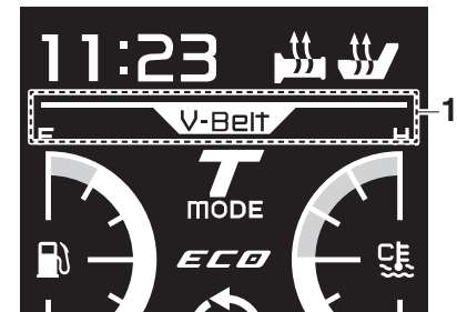
1. V-belt replacement indicator “V-Belt”
