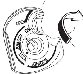
Insert the keyhole shutter key into the keyhole shutter receptacle as shown, and then turn the key to the right to open the keyhole shutter.
