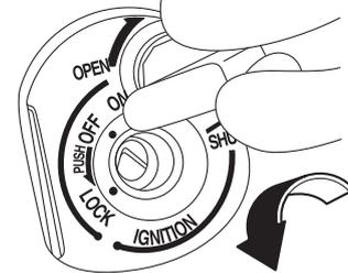
Insert the keyhole shutter key into the keyhole shutter receptacle as shown, and then turn the key to the left to close the keyhole shutter.
