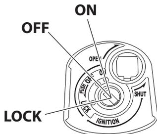
The main switch/steering lock controls the ignition and lighting systems, and is used to lock the steering. The various main switch positions are described below.
