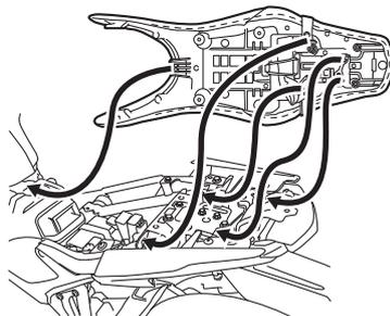
2. Push the rear of the seat down to lock it in place.
