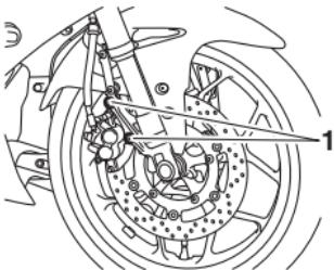
1. Brake caliper bolt
