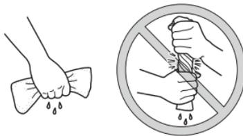
4. Apply oil of the recommended type to the entire surface of the sponge material, and then squeeze the excess oil out.
